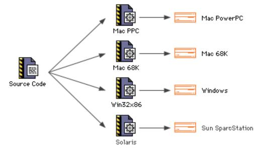
Java bytecodes cannot run directly on any real machine. On the other hand, the Java bytecodes created by the CodeWarrior Java compiler can be interpreted to run on *any* platform that has a bytecode interpreter (BCI). You write the code once, compile it once, and then you are done.
